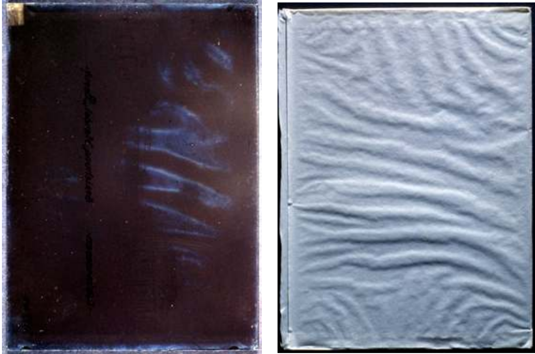
Figure 21. Silver gelatin glass negative. Schweizerische Landesaussstellung 1914. Bern State Archive. Stripes of silver mirroring (a) matching the creases of the glassine envelope (b) in which the plate was stored.
