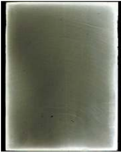
Figure 10. Silver mirroring edge pattern artificially created exposing a single plate in the incubation chamber without ventilation.
