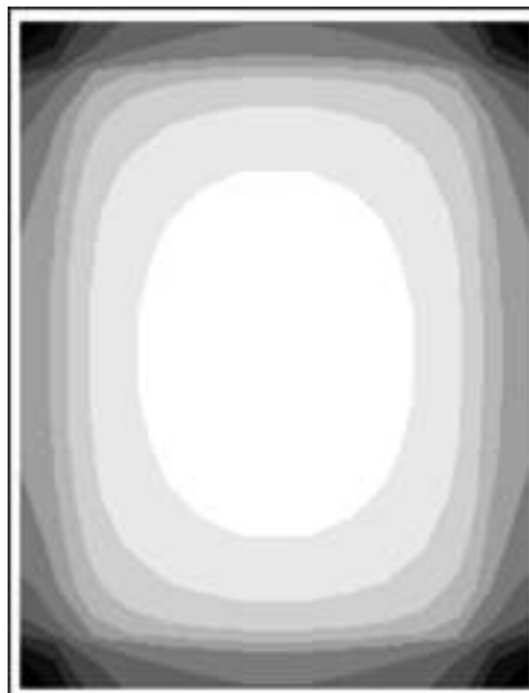
Figure 4b. Contour plot of the gas absorption rate on a rectangular plate freely exposed to environmental gases. The value of the gas absorption rate is proportional to the grey density.
