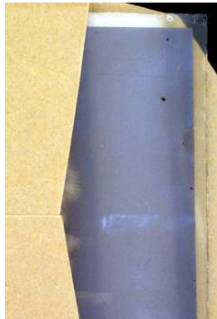
Figure 20. Silver gelatin glass negative. Hö Nachlieferung, plate 42, Basel State Archive. Stain of silver mirroring connected with the seam of the envelope. For purpose of showing this effect, the plate is shifted to the right.
