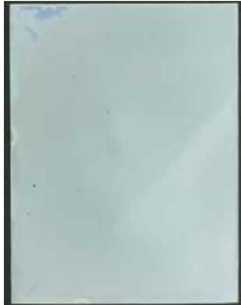
Figure 11. Homogeneous silver mirroring artificially created exposing a single plate in the incubation chamber with continuous ventilation.
