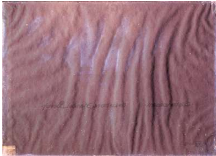
Figure 4. Superimposition of the images of the negative shown in Figure 1 and of the glassine envelope in which the plate was stored.
