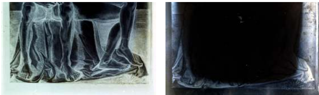
Figure 8. Silver gelatin glass negative. Cueni study collection (~1910). The comparison between the photograph in transmission (a) and in reflection (b) shows that the silver mirroring intensity is proportional to the image density.
