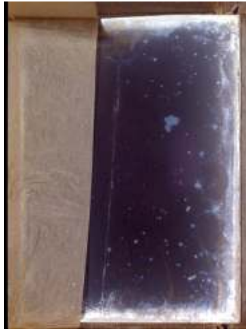
Figure 14. Silver gelatin glass negative (Courtesy of S. Dobrusskin). A straight line of silver mirroring is formed along the edge of the storage glassine paper. For purpose of showing this effect, the plate is shifted to the right.
