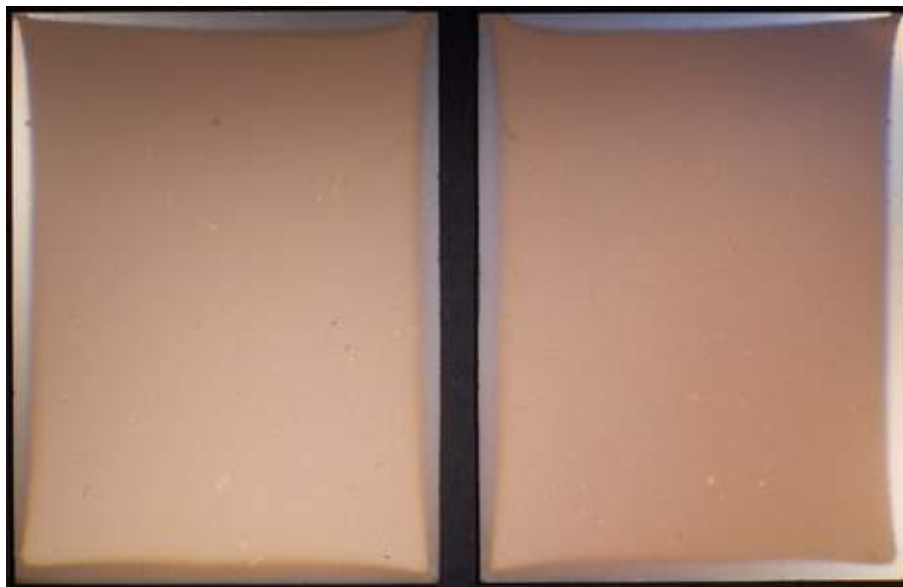
Figure 10. Pair of non-processed silver gelatin glass negatives Cueni study collection (~1910). The silver mirroring edge pattern is exactly the same on the two plates.
