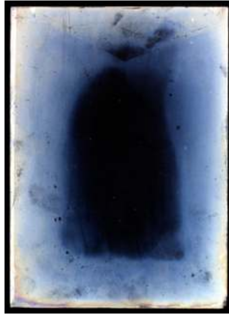
Figure 3. Silver gelatin glass negative. Cueni study collection (~1910). The mirroring stain is wide, partially obscuring the image.
