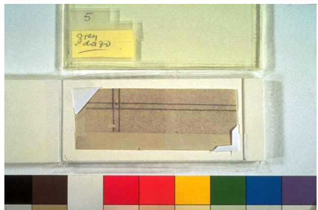
Fig. 8. Diazo example after testing equivalent to seven venues
