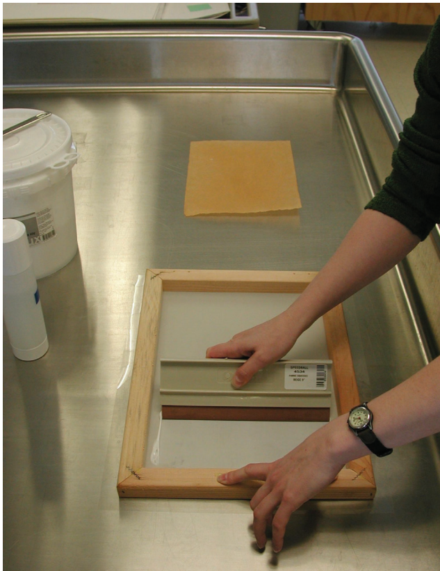
Fig. 1. Squeegeeing through silkscreen onto polyester film
