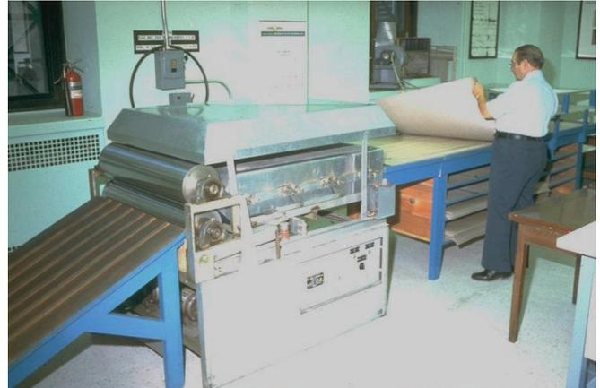
Fig. 3. Arbee rolling lamination press, NARA
