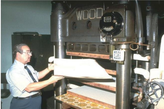
Fig. 2. Wood hydraulic laminating press, NARA
