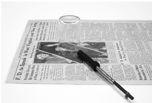
Fig. 3. This newspaper was laminated in 1936 during the first run of the presses at the National Archives. The volatile plasticizers in the lamination film were sampled by placing a beaker upside-down on the document and slipping a SPME fiber underneath the lip of the beaker. The PDMS/DVB fiber was exposed for 40 minutes.
