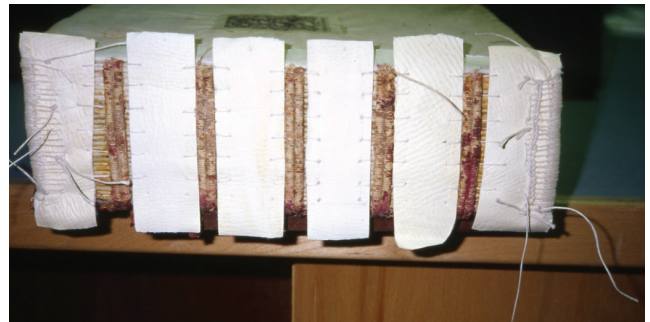
Fig. 4. New spine lining attached to stays via long stitches
