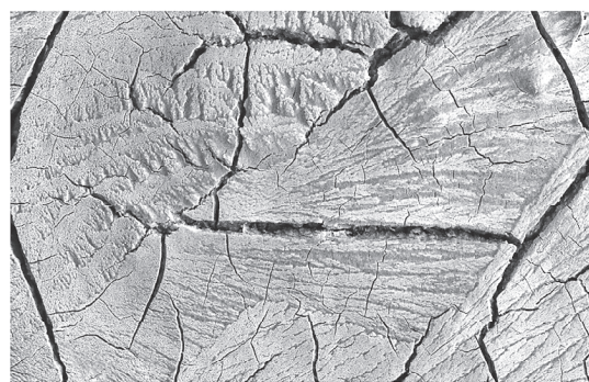
Figs. 8c–d. 1: 1.52: 0.25 (weight ratio of iron (II) sulfate: gallnuts: gum arabic)
