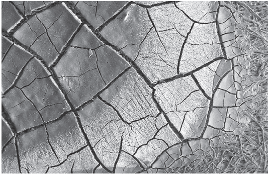
Figs. 9a–b. 1:2.0:0.5 (weight ratio of iron (II) sulfate: gallnuts: gum arabic) after artificial aging by humidity cycling at constant room temperature.
