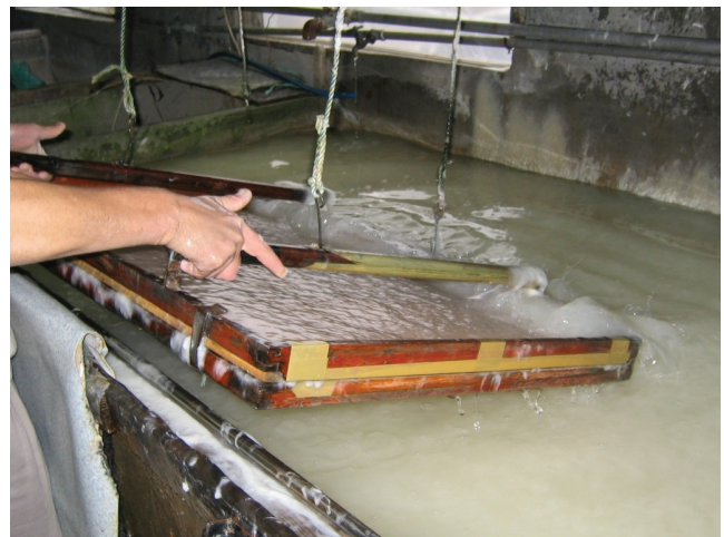
Fig. 16. Excess fibers are tossed off top of mold. Photo courtesy of FIDES.
