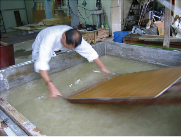
Fig. 8. Initial dip of webal method of sheet forming. Photo courtesy of FIDES.
