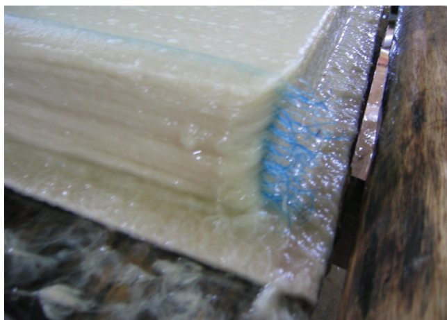
Fig. 19. A blue string is used to separate sheets on post of wet sheets. Photo courtesy of FIDES.
