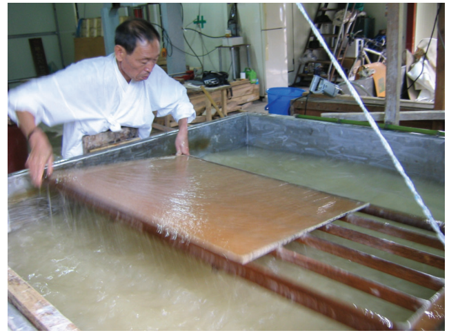
Fig. 11. Swinging mold to remove excess fibers. Photo courtesy of FIDES.
