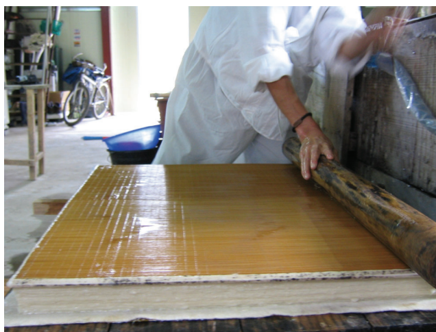
Fig. 18. Rolling log across post of wet sheets to remove bubbles. Photo courtesy of FIDES.
