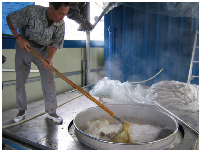
Fig. 3. Cooking white bark with alkali to remove non-cellulosics. Photo courtesy of FIDES.
