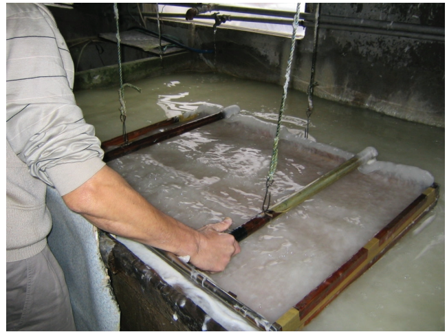
Fig. 15. Shaking mold front to back while water drains. Photo courtesy of FIDES.
