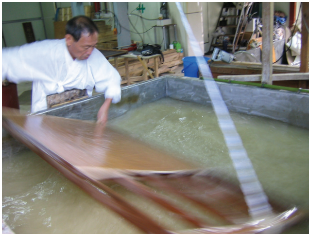
Fig. 10. Dipping left side of the mold into vat. Photo courtesy of FIDES.
