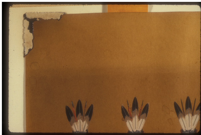
Fig. 3. Plastic photo corners, charred and melted
