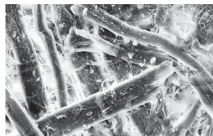
Fig. 9. Paper T0, SEM image of paper surface, 1000x magnification.
