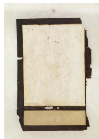
Fig. 8. Paper T7, combined calcium phytate/calcium bicarbonate treatment, lining with wheat-starch paste, after aging.
