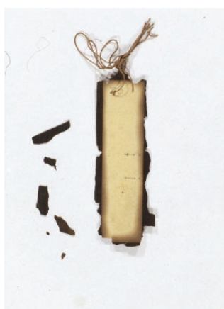
Fig. 3. Paper T0, untreated control after aging.
