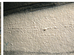
Fig. 11. Highlight area with extensive flaking of the photographic emulsion (c. 6x magnification).
