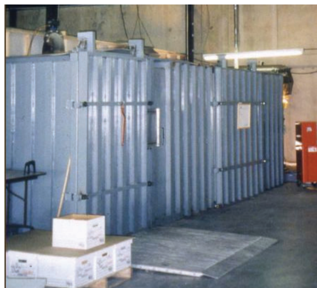
Fig. 4. Vacuum freeze drying chamber, Belfor USA
