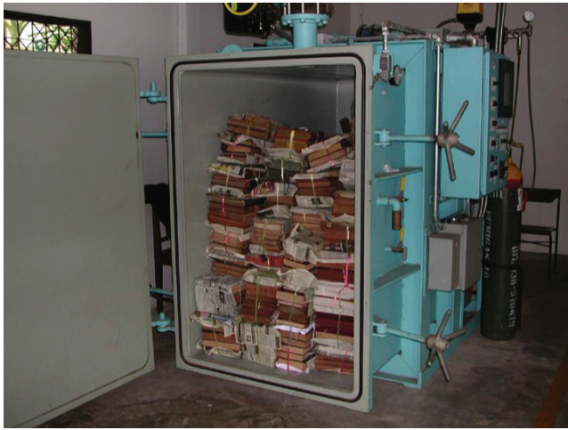
Fig. 11. Books in ethylene oxide chamber, Czech National Archives
