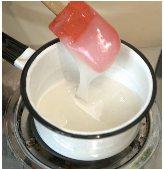
Fig. 6. Bubbles develop and elongate. Paste takes on a slightly gelatinous or rubbery quality and becomes more opaque.
