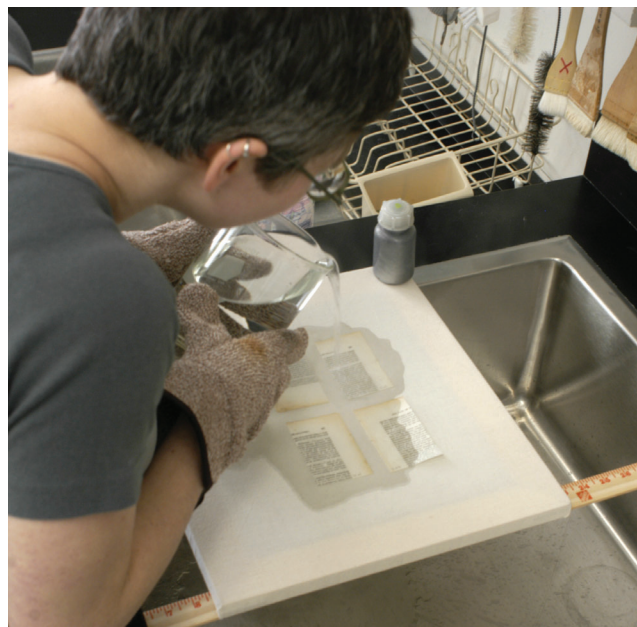
Fig. 5. Pouring boiling water over the samples from 1836
