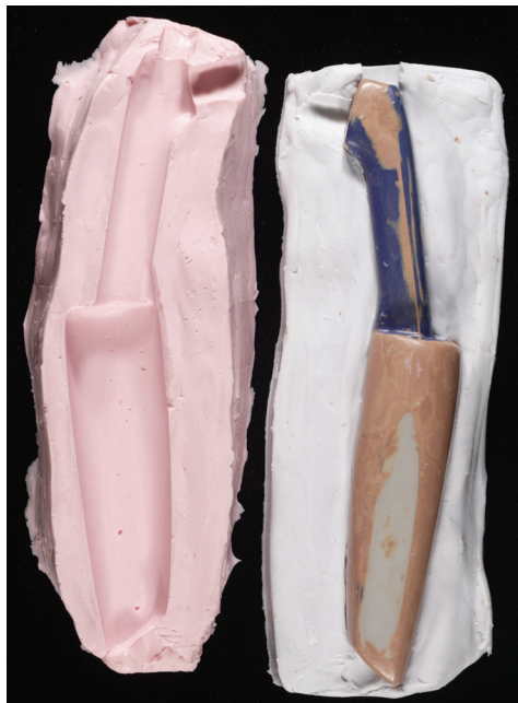
Fig. 5. Cured silicone rubber mold with prototype
