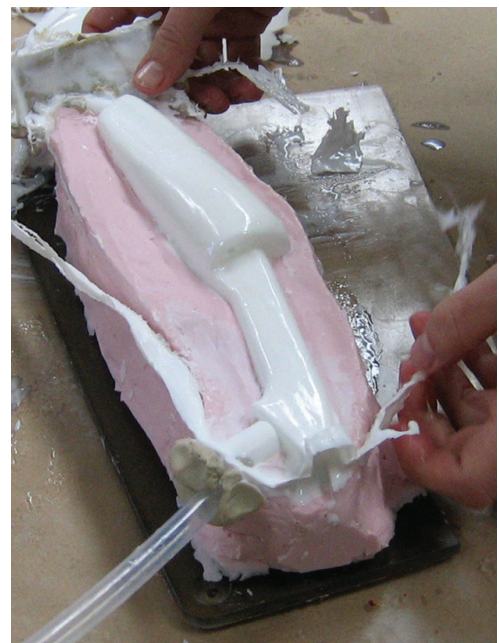
Fig. 6. Handle cast in polyurethane resin
