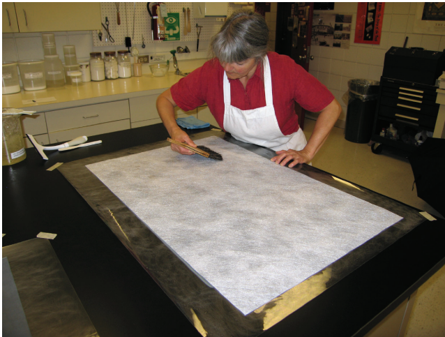
Fig. 12. Brush out the tissue through Reemay from the center outwards
