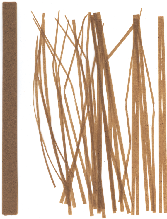
Fig. 1. Trial samples of remoistenable mending tissue for papyrus. These mending strips were made over the winter in very dry conditions, which caused the paper to curl. This turned out to be an advantage: I flattened the roll and vertically cut narrow strips ready to use. Left: the remoistenable Japanese paper rolled up into a tube and flattened; right: cut strips measuring 1–3 mm wide (leaving the top of the tube uncut makes the strips easier to handle and store).
