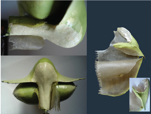
Fig. 19. Damaged sepal in gelatin with delaminated paint. Lycopodium clavatum L., Lycopsidea. R. Brendel, Berlin, no. 193
