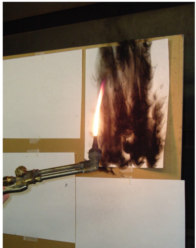
Fig. 3. Making soot samples with oxy-acetylene welding torch
