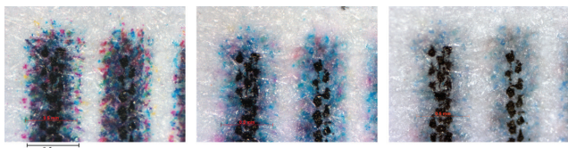
Fig. 4. Photomicrographs of printed black lines before (left) and after (center) fixing with Cartafix NTC, and after immersion washing (right). Note the marked bleeding and fading of colored inks after fixing and further fading after washing, while the black ink remained in place
