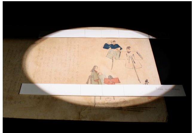
Fig. 2. The Recording Verification Target (bottom strip) and the Reproducibility Target (top strip) during the recording of a test document
