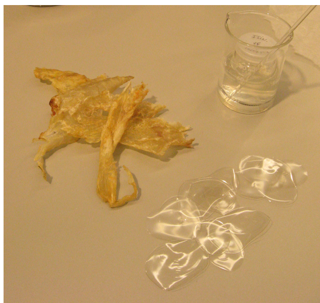
Fig. 12. Isinglass in various forms: (clockwise from upper left) desiccated raw bladder, in solution ( bain-marie ), and dehydrated purified disks
