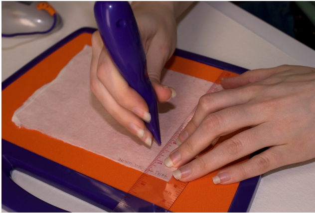
Fig. 12. Using the Crayola™ Cutter to create a series of perforated lines on a medium-weight Japanese paper to be used as detachable hinges
