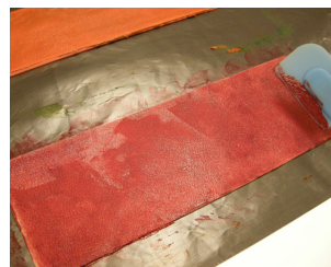
Fig. 5. The acrylic blend is applied to the silicone mold with a wide spatula to create a uniform film.
