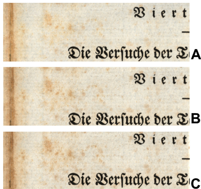
Fig. 3. Photos of artificially aged original document before aging, after 2 and after 5 aging steps simulating as many months of exhibition in a suitable environment
