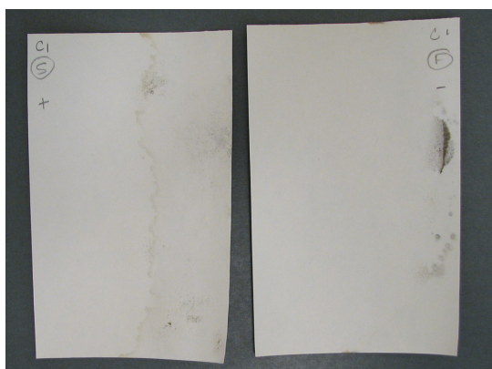
Fig. 3. Clear Spring offset paper, image taken at day 40. Similar mold growth was observed on Bookkeeper treated and untreated papers of this paper type. In this image, Bookkeeper treated sample is on the left and untreated sample on the right. Tidelines more distinct on Bookkeeper treated samples
