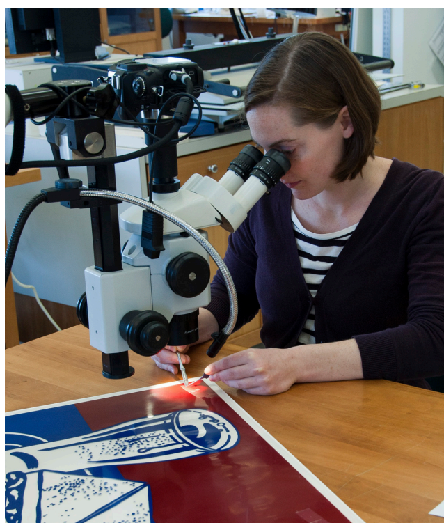
Fig. 3. Sampling the tape carrier under the microscope
