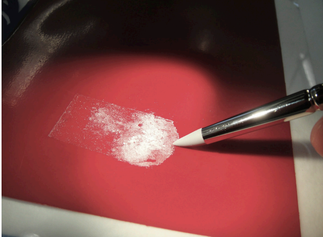
Fig. 4. Removal of tape adhesive residues with cellulose powder and a Colour Shaper tool
