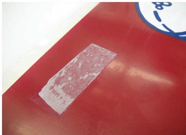
Fig. 2. Filmoplast tape attached to the ink layer on the verso of one of the prints (Harvard Art Museums, M14194)
