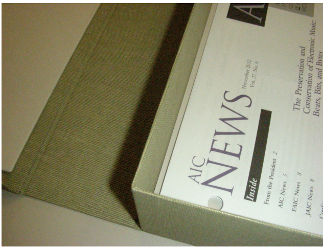
Fig. 2. This thin aluminum wall, laminated with acid-free paper and covered with starch-filled buckram, measured 0.045 in. thick, whereas a double wall of binders' board would have been 0.140 in. thick and weighed much more.
