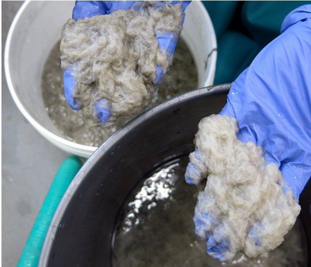
Fig. 21. Pulp prepared by cooking with soda ash, washed and beaten once (upper left); and washed and beaten three times (lower right). Courtesy of Anne Covell.
