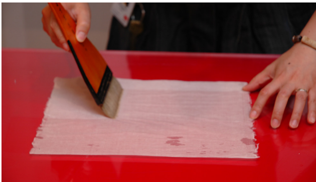
Fig. 8. Uda paper was sized with alum gelatin solution (3% gelatin and 0.5% alum) using 1–2 brushed applications.
