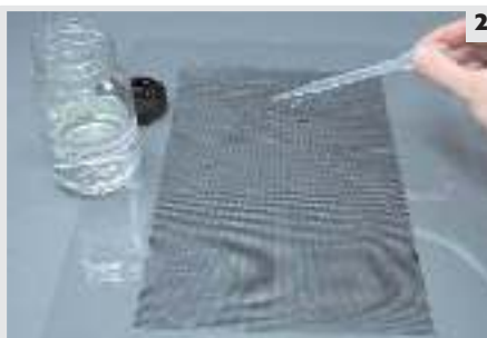
2 Use the pipette to load the screen with the gelatine.
