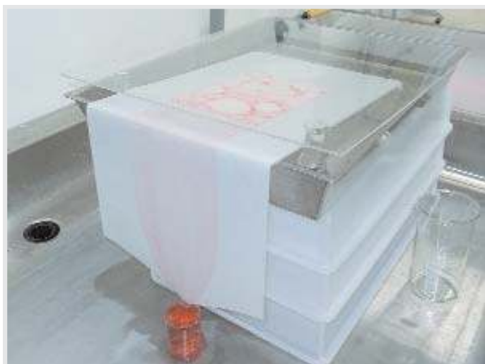
2 The treatment of a sample of blotting paper on the capillary unit. The red dye simulates the water-soluble degradation products that washing is meant to remove.
