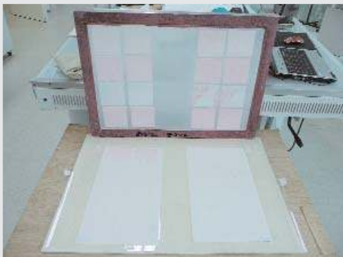
8 Changing of the soiled Paraprint OL 60 (left) and blotting paper (right). The screen is standing on its edge for the photograph, before being moved to the second table.
