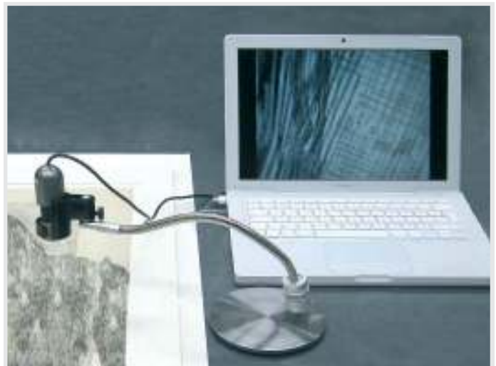
2 Mounting the Dino-Lite® Digital Microscope in a stand for keeping distance to a surface. Photos: Birgit Reissland.
