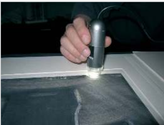
1 The use of the Dino-Lite® Digital Microscope for examination of a drawing in direct contact.
