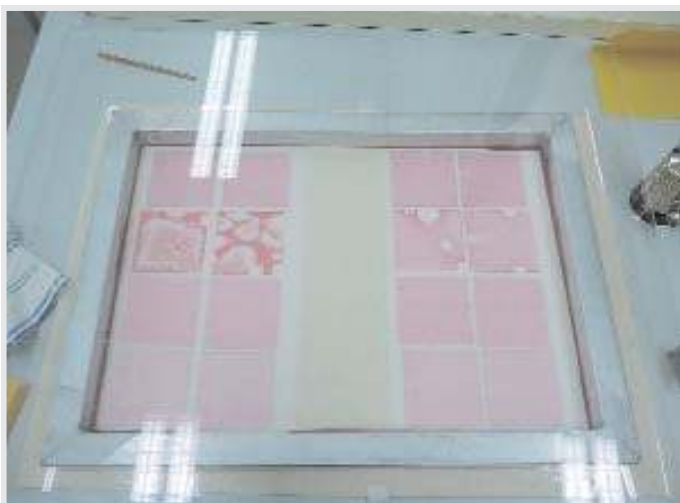
7 Paraprint washing (left) and blotter washing (right) the samples on one screen.
