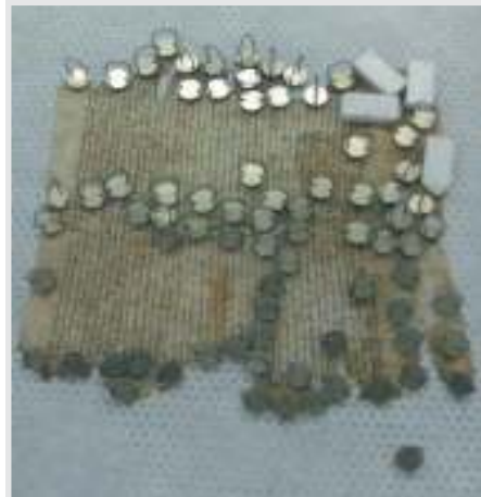
6 Document clamped with magnets: top view.
