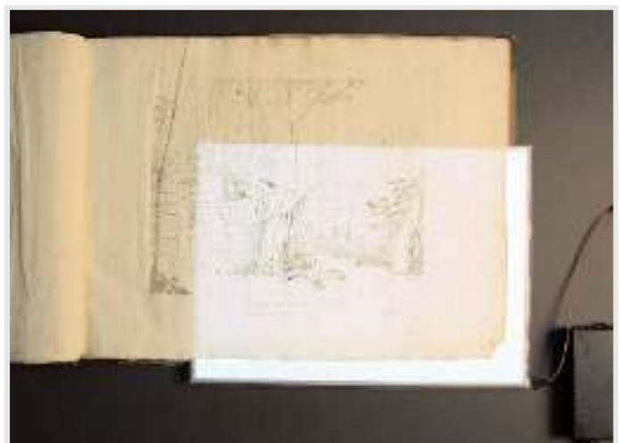
2 The Electroluminescence Panel in use in the examination of an album sheet. All Photos: Dionysia Christoforou. © Rijksmuseum Amsterdam.
