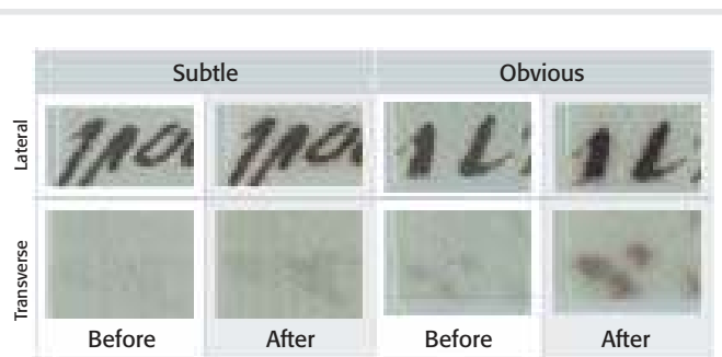
6 Samples with subtle and obvious ink migrations after re-sizing.
