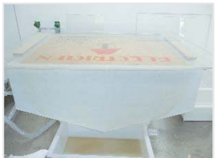
9 Washing the gouache on the capillary unit. Discolouration washed out of the object can be seen traveling through the Paraprint OL 60 and in the container below.
