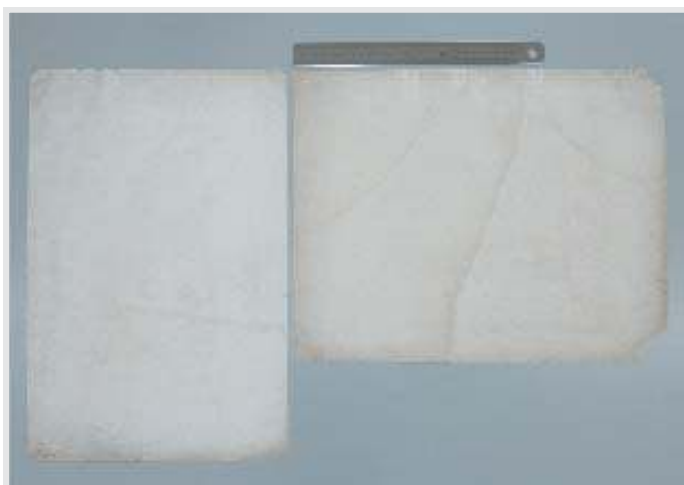
10 Verso of two prints from the same series. Left was washed on the capillary unit, right was immersion washed.
