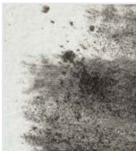
Microscope view of charcoal strokes on paper, x120. © L Sauvage.
