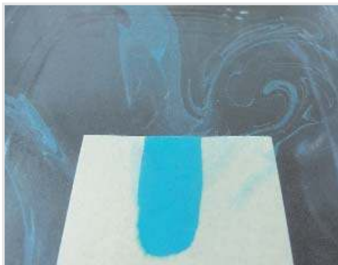
1 Water-sensitive media: a sample of paper with blue gouache paint during immersion washing. The loss of pigments is clearly visible.
