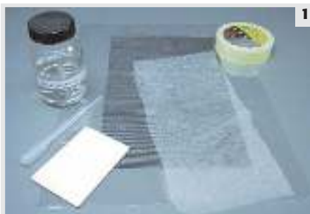
1 Tools and materials for remoistenable tissue. The purpose of the screen is to control the thickness and homogeneity of the gelatine layer.
