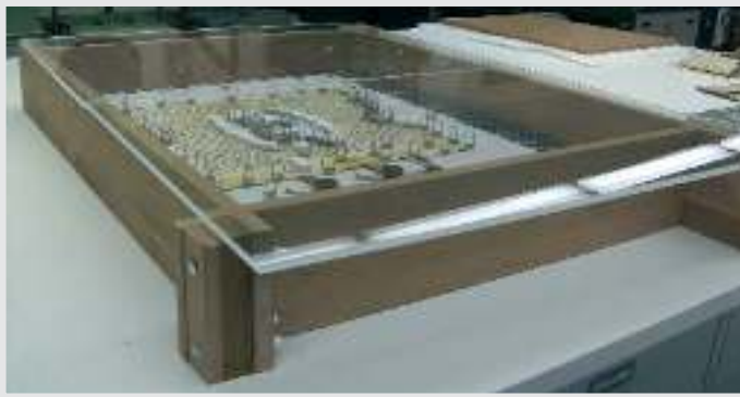
3 Document on magnetic frame inside humidifying chamber (cedar-wood with Plexiglas cover).
