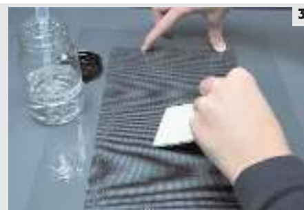
3 Spread the gelatine with the squeegee and even out the gelatine, add more gelatine if necessary, all of the surface of the screen should be filled with gelatine.
