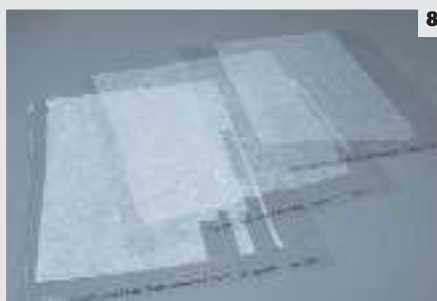
8 Prepared remoistenable tissue, different - paper weight. Note that name, weight, supplier of the paper, the adhesive used as well as date of manufacture of the tissue are noted on the margin. Some have already been used in repairs. You can keep these sheets for a long time in a dark and dry place.
