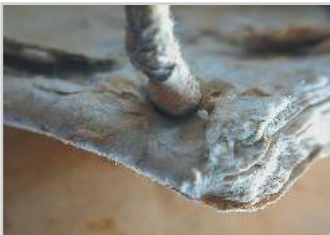
8 Particular of a board spine edge: a single piece of a laminated board folded at the centre [11].
