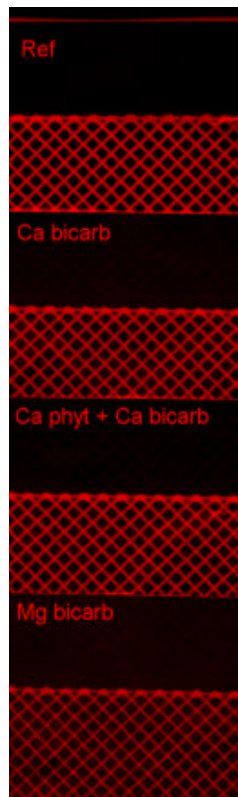
Figure 7. Discolouration of 12 days aged standard reference papers - clearly visible is the strong yellow discolouration of the magnesium bicarbonate treated paper, while the calcium bicarbonate and the calcium phytate / calcium bicarbonate treated papers are only insignificant yellowed in comparison to the untreated reference. Due to artificial ageing, the ink of all samples darkened with the exception of inks treated with magnesium bicarbonate. Tis inks changed to a lighter brownish colour.
