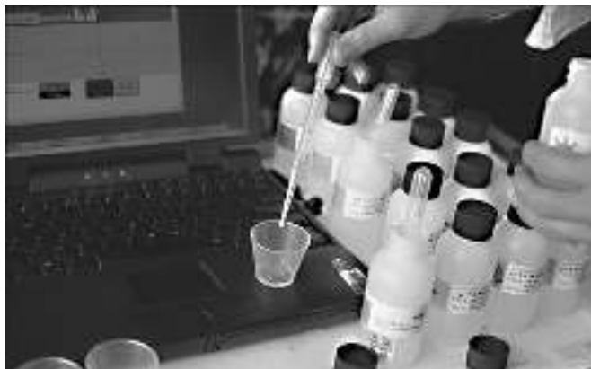
Figure 8. Detail of pipettes and measuring cups used with the concentrated stock solutions.
