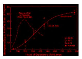
Figure 3. Evolution of butyric acid from PVBs exposed to UVA Lamps (Feller et al. 2007)
