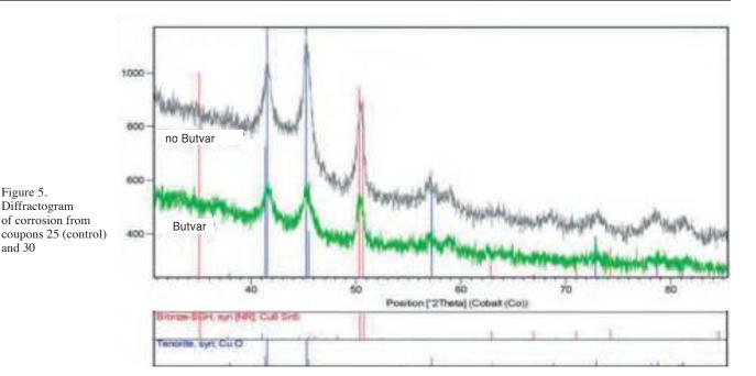
Similarly, XRD confirmed that tenorite was produced on both types of coupons, which suggests that the copper was oxidized in each case via the same corrosion mechanism (fig.5).
