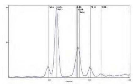
sources but typically W, Rh, Mo, Ag, and Re) enter the sample and elastically bounce off the atoms within that sample with no loss of energy, and are detected as the characteristic energy from the source anode. This results in spectral peaks at the characteristic emission energies originating from the tube source.
