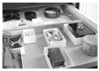
Fig. 6 Acid vapors released from degraded plastic materials (center) have corroded a metal pan (photo center top) and a metal box (photo lower right) in the same drawer.
