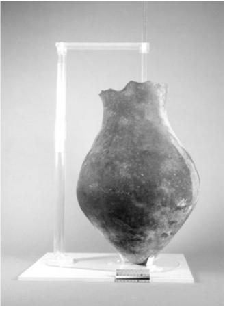
Because of the relatively thin dimension of the tubing walls, the nylon fasteners chosen for adjusting the height of the main column quickly degraded due to the pressure on the few threads that were in use when tightened. These were replaced with steel fasteners for durability and the nylon fasteners would only be used during x-ray analysis.
