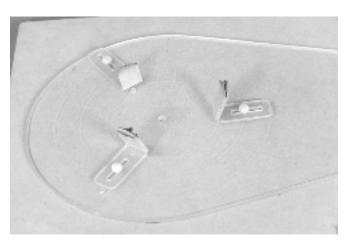
In some instances, it was found that the stops gave sufficient stability to the pot that there was no need to use the upper support, thus allowing for photographs with no visual intrusion into the pot mount.
